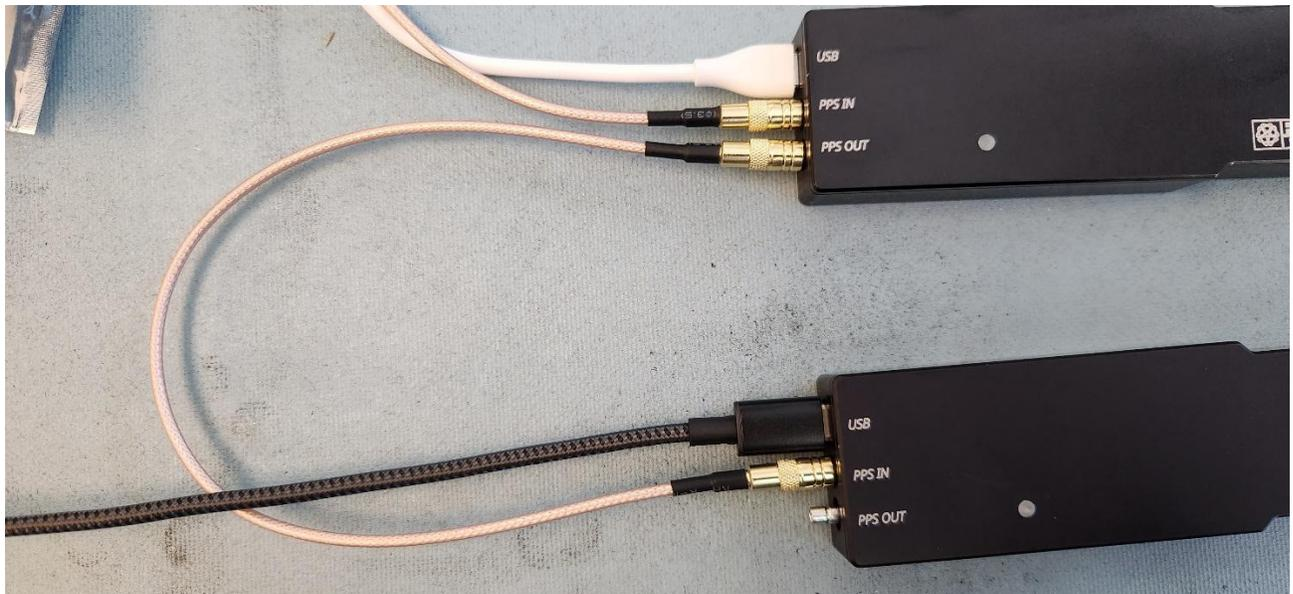
**Figure 3 - PPS Connections**
